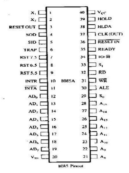
The 8085A is a complete 8 bit parallel central processor. It requires a single +5 volt
